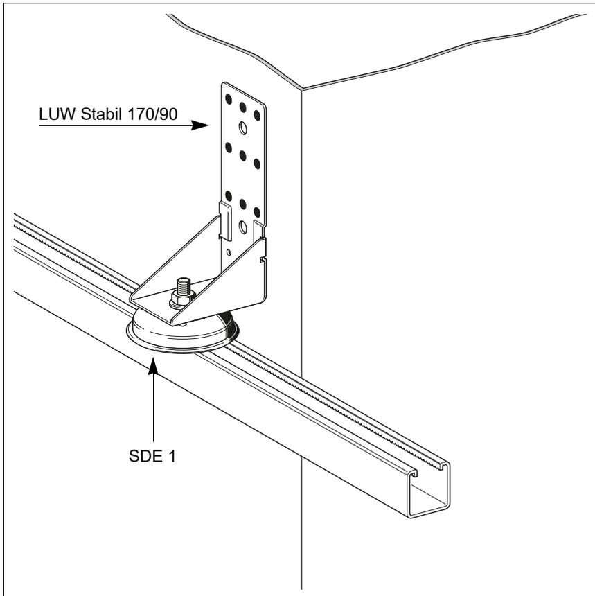
Fixing vertical ducts on a suitable support (horizontal channel).
