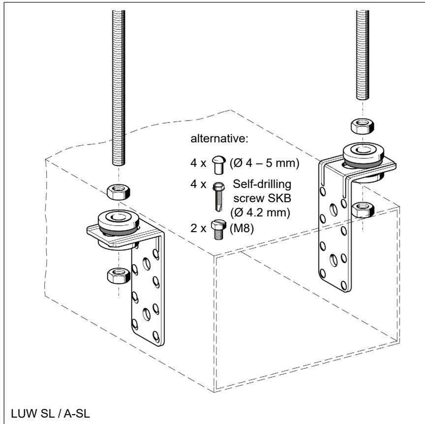
Fixing of the Ducting Angle LUW to the duct by 4 to 8 steel rivets or tapping screws.
